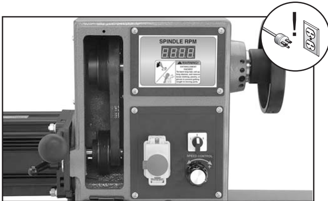
Figure 29. Belt access panel removed.
